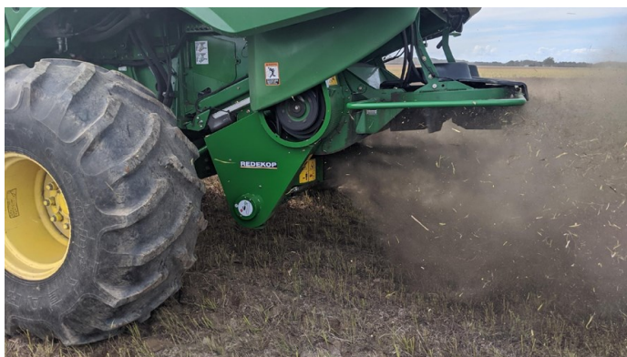
Redekop Seed Control Unit in operation during soybean harvest in Virginia.
